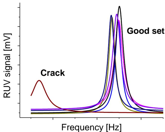
Figure 1: Deviations of RUV peak parameters caused by a crack
