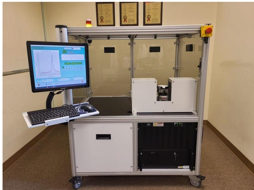
**RUV system for ZrO<sub>2</sub> discs**
