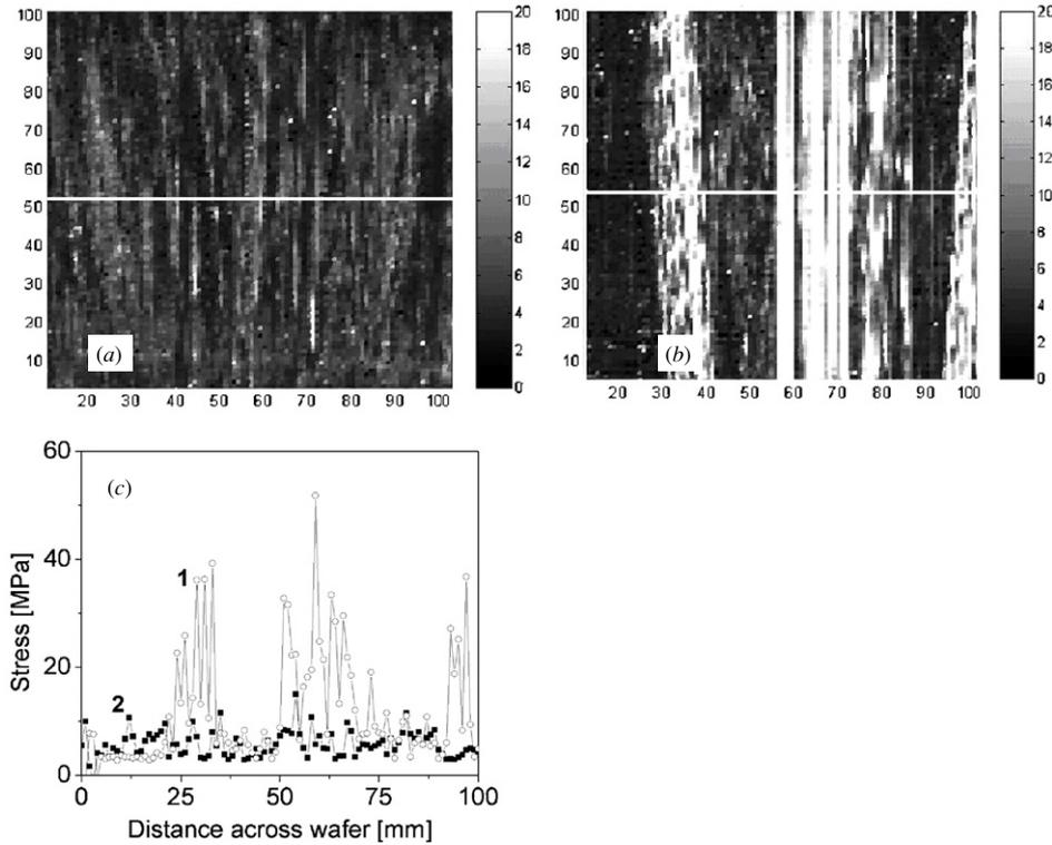
**Figure 5.** Stress mapping using the infrared polariscopy: (a) a low-stress wafer (number 16) and (b) high-stress wafer (number 22). Contrast bar is (MPa) values. The horizontal lines on the maps indicate the position of scan lines we have shown in (c), where data (1) correspond to wafer number 22 and data (2) to wafer number 16.
