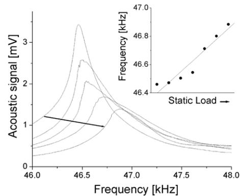
**Figure 9.** Frequency curves of the 46.5 kHz resonance vibration mode at different load values using five-point bending test. The arrow shows the direction of the load increase. Inset represents the resonance frequency peak upward shift with the increase of the static five-point bending stress.
