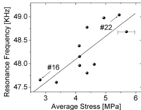
**Figure 8.** Experimentally measured frequencies of the resonance longitudinal vibration mode versus average stress by the infrared polariscopy technique in a set of 100 mm  $\times$  100 mm EFG wafers. Two wafers with low (number 16) and high (number 22) average stress are indicated in the graph. Note that the error bar for average stress is estimated as 0.6 MPa due to a sensitivity limit of the polariscopy set-up.
