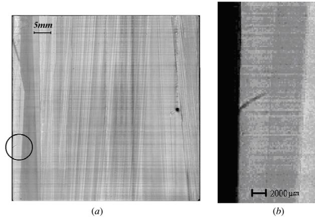
**Figure 4.** SAM image of the 100 mm  $\times$  100 mm EFG wafer with periphery crack: (a) image of the entire wafer, the crack is circled at the wafer's periphery; (b) zooming area of the crack with 5  $\mu$ m step.
