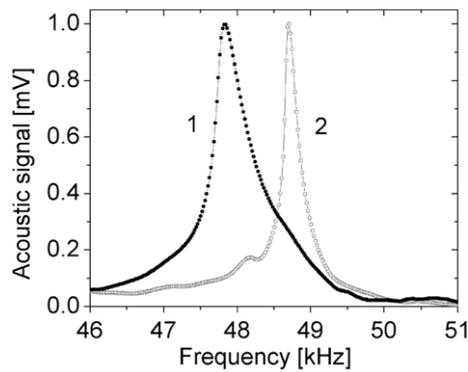
**Figure 7.** Normalized by intensity frequency scans at the principal maximum on two EFG wafers: (1) low-stress wafer number 16 with average stress of 5.6 MPa; (2) high-stress wafer number 22 with average stress of 2.8 MPa.
